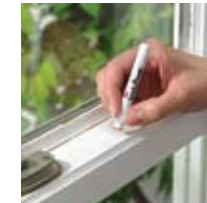
3M™ LeadCheck™ Swabs only turn red when lead is present. So there are no false positives from your customer's point of view.
